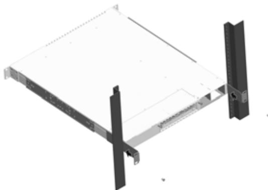
Slide Rear Brackets into Side Rails and Mount
